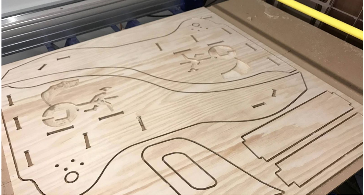
Figure 8: Cutting out the rickshaw pieces with the Shopbot
