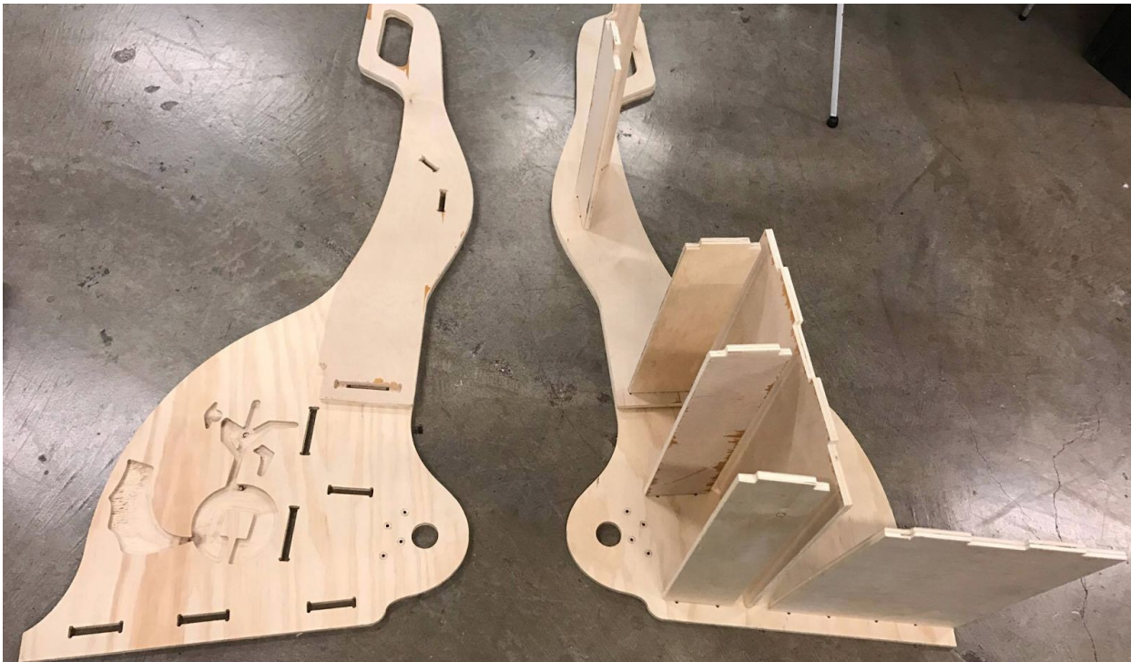
Figure 9: Assembling rickshaw pieces with wood glue and wood screws
