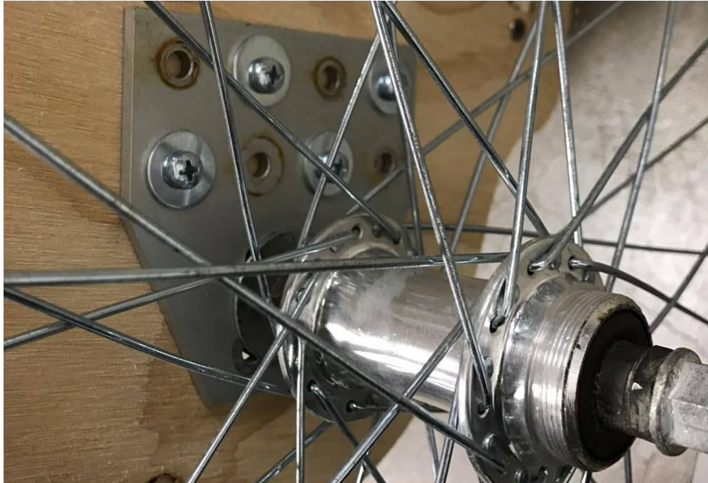
Figure 11: Aluminum plates used as interface between the wooden pieces and wheels
